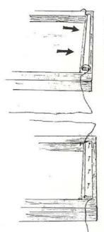
2) Roll thin battens (ideally 25mm x 12mm) timber battens tightly into the polythene and nail to the door/vent frame as shown. Roll and stretch the polythene in the battens as much as possible before nailing to obtain a neat, tight finish. Fix battens in sequence shown 1,2, etc.
