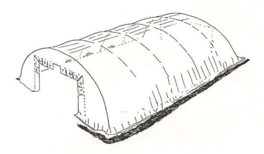
1) Tightly batten (as shown on previous page, A, B,C, and D) around the top corners of the Door Frame.
