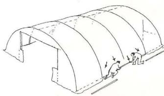
1) Clad house in normal way from the centre outwards and ensure the polythene sheet is aligned correctly on the structure, stretch the polythene lengthways as previously described.
