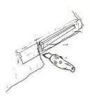
3) With a sharp knife carefully cut the rolled up polythene at one of the butt ends of the batten (hold the loose polythene securely to prevent a gust of wind ripping your cut further up the sheet). Roll another batten next to the first and so on until you are within 2.4m of the end hoop.
